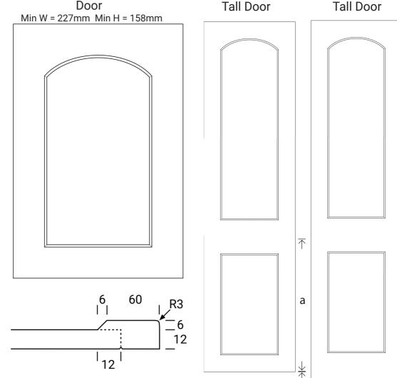
Max door H = 2400mm Min H with rail = 500mm
